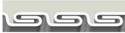
Interlocked Design 1-1/2" through 4" with no bonding wire
